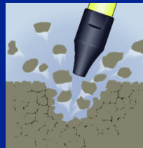
The crevices explode from the energy built-up from the forced compressed air, crumbling the soil and leaving it dry for easy vacuuming and backfilling.
