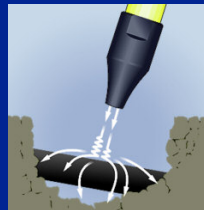
As the cable or utility is exposed, the air stream hits its non-porous shielding, compresses, and harmlessly dissipates in the soil that surrounds the cable.
