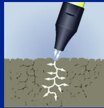
VACMASTERS supersonic air stream, delivered through its Air-Tec™ nozzle at 150–220 psi, is forced into these microscopic pockets.
